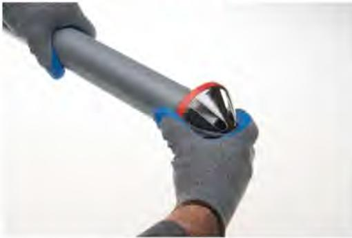
Burrs and filings can prevent proper contact between the pipe and fitting and may put undue stress on the pipe and fitting assembly. Burrs and filings must be removed from the outside and inside of the pipe. A chamfering tool or file is suitable for this purpose.
